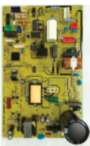
MCC-1626 : Control, LED check code, miss-wiring protection circuit.
